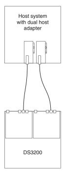
Figure 29. Dual-controller direct-attached connection to two HBAs in the same host (redundant host connection)
